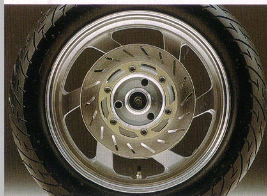
The sixteen-inch front wheel is actually a slotted aluminum disc.
